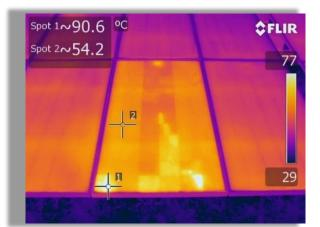
Infrared image showing hotspots on electrically isolated cell sections
