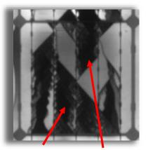
Electroluminescence image showing electrically isolated cell sections
