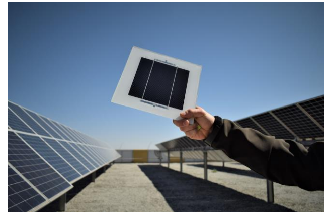
Encapsulated mini-modules and single-cells are finding their place in outdoor testing.
